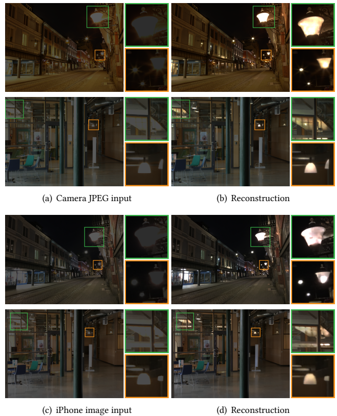
Fig. 11. Reconstruction from Canon 5DS R camera JPEG (top). The examples are the same as in Figure 9, but with the camera set to store JPEG, applying unknown image transformations and compression. Reconstruction can also be performed with hand-held low-end cameras, such as the iPhone 6S (bottom), where the input image is more degraded.
