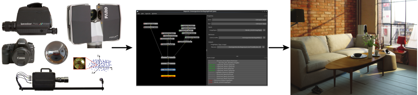
Figure 1: Multiple capture devices (left) are used to scan a real-world photo studio. The resulting data and processing software is organized by the Depends workflow management application (center), to create a computer graphics rendering of a real-world environment (right).
